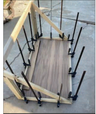
Here we see the Douglas fir shell being glued and clamped. The first of the walnut veneered plywood panels is being attached to the frame.
