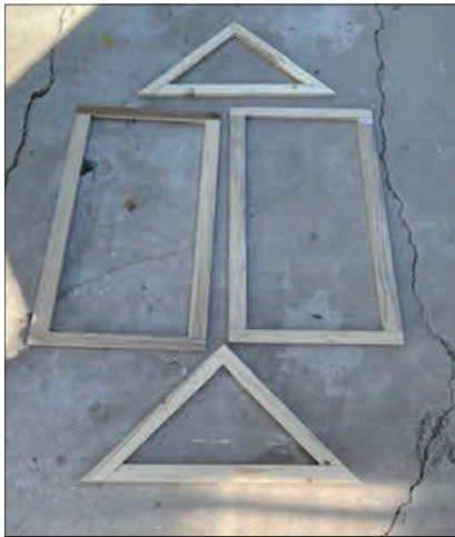
This is the lay out of the Douglas fir 'bones' of the corner cabinet pre glue-up.
