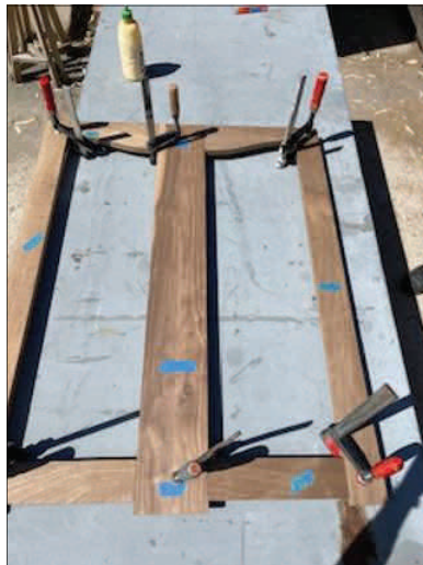
This image shows the solid walnut door frames being glued and clamped prior to being shaped with a router to the shape and dimensions of the stained glass, that will be inset into the frames.
