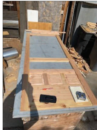
Unpainted screen door assembled with all panels in place and screen installed.
